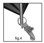
4. Raise the frame: Start at either end and insert the ridge pole into the hub. Walk to the opposite end and grasp both the ridge pole and the second hub. Push/curve the poles until the ridge pole fits securely into the second hub. See fig. 5.
